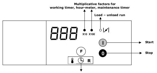
Visualization temperature - working hours - Maintenance timer - Reset
