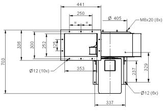
Duct inlet diameter 400 mm
